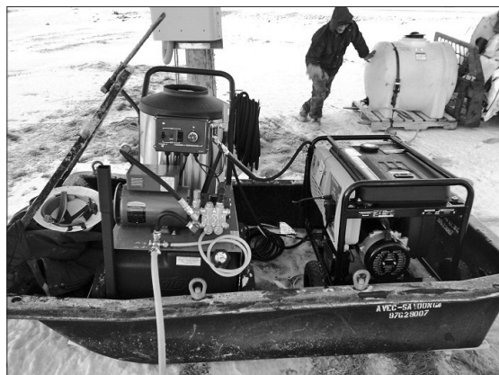
A power washer, hooked up to a portable generator and water container, was used to remove frozen salt residue coating the power equipment. A snowmachine towed the heavy sled.
